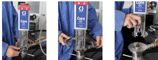
1. Loosen T-handle 2. Open Pump Clamp 3. Slide Electric Motor to Remove
